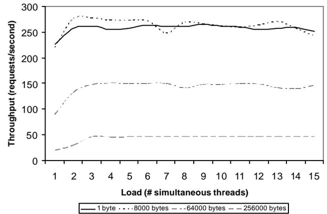
Fig. 4. Throughput (req/sec) vs. load for different file sizes (HTTP 1.0)
