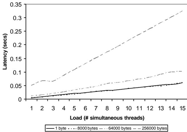
Fig. 5. Latency (secs) vs. load for different file sizes (HTTP 1.0)
