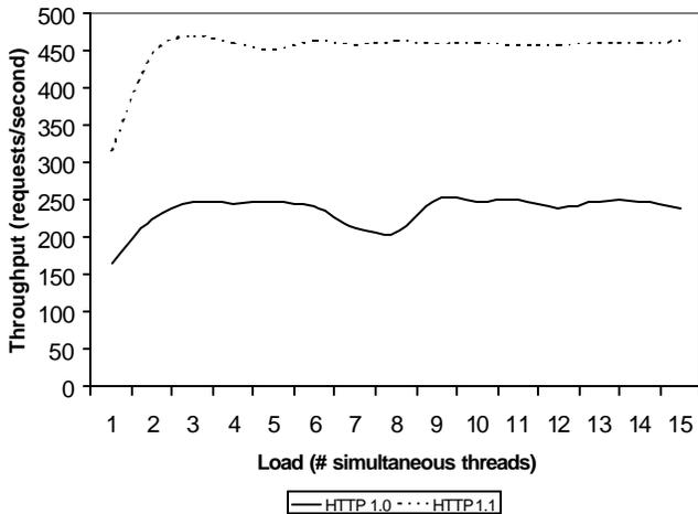
Fig. 1. Throughput (req/sec) vs. load for 8kb file size
