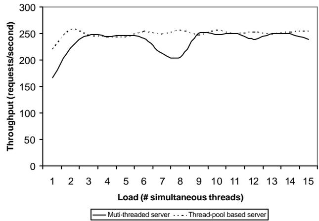
Fig. 6. Throughput (req/sec) vs. load for 8kb file size
